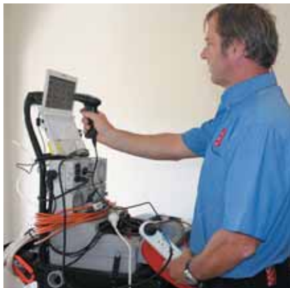
The use of a Portable Appliance Tester remains one of the most comprehensive and efficient methods of ensuring an item’s electrical safety.
